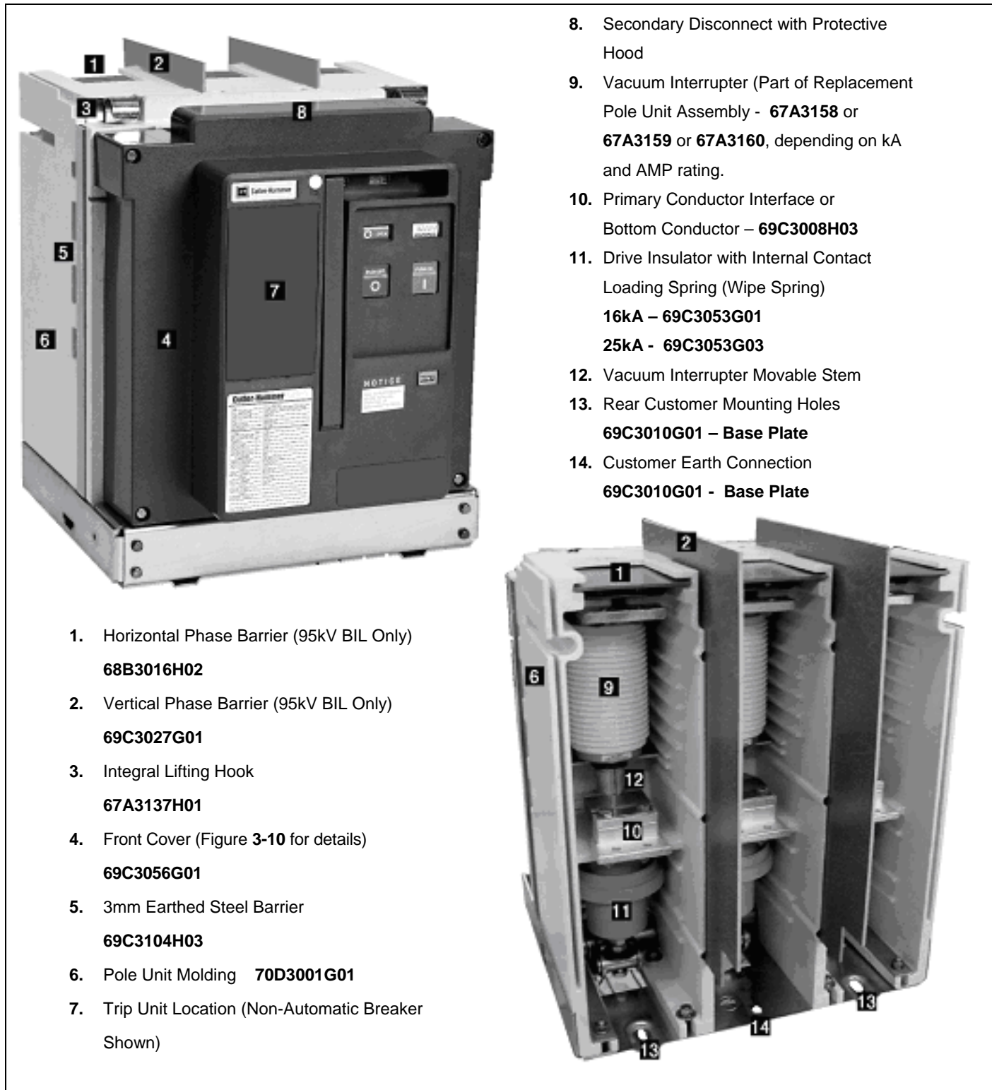
Figure 3-5 Front and Rear Views All T-VACR Fixed (except 25kA, 2000/2500A and all 31.5/40kA)
